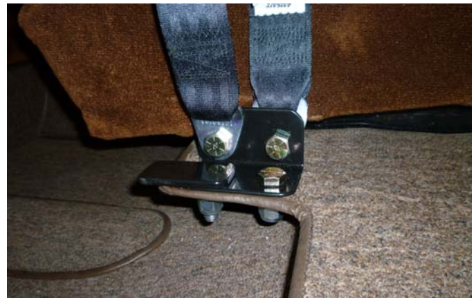
The L-bracket for the inboard belts is attached to the front seat back rest plate located between the front two seats.
