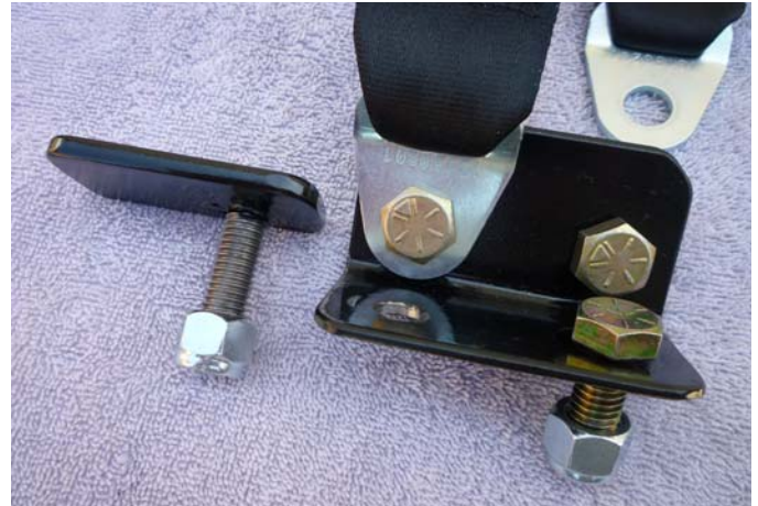
The center belt L-bracket attaches to the passenger side of the seat back rest plate, The bracket at left attaches to the L-bracket to provide a platform for the back inboard passenger seat back peg to rest on.
